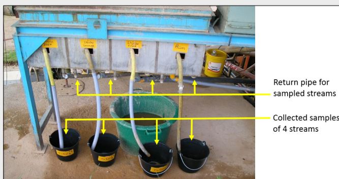
Figure 9. Simultaneous sampling of four slurry streams with mutual sampling proportionality.
